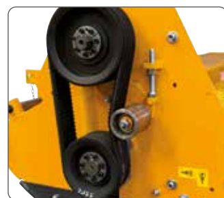
Trasmissione a cinghie dentate (4 cinghie SPBX). Toothed belt drive (4 SPBX belts).
