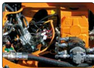
Impianto a pistoni a circuito chiuso. Closed circuit piston pump and motor.
