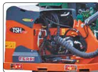
Impianto a pistoni a circuito chiuso (TSH Power). Closed circuit piston system (TSH Power).
