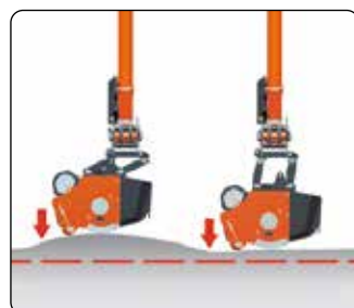
Sistema autolivellante Self-levelling device.
