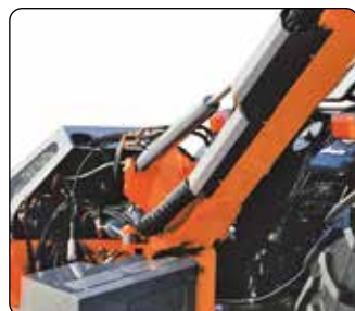
SAB Sistema antiribaltamento. SAB system Roll-over protective kit with inclinometer.
