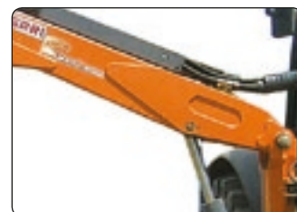
Bracci in WELDOX 700. WELDOX 700 drop forged arms.
