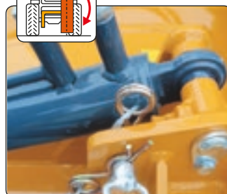
Perno per blocco meccanico in trasporto, (no catene, no staffe). Mechanical locking pin for transport (no chains, no brackets).
