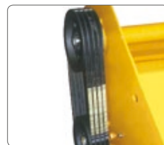
Trasmissione a cinghie dentate (4 Cinghie SPBX). Toothed belt drive (4 SPBX belts).
