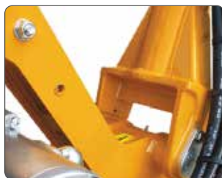
Elementi stampati. Drop forged brackets.
