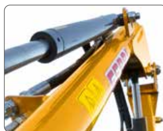
Bracci a sezione circolare High Torsion Resistance. Arms with circular section H.T.R. (High Torsion Resistance).
