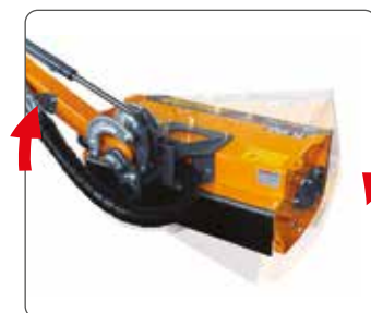
Sistema Floating. Floating head system.
