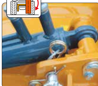
Perno per blocco meccanico in trasporto, (no catene, no staffe). Mechanical locking pin for transport (no chains, no brackets).
