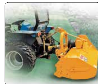
Versione MTR Per trattori con guida reversibile MTR version For tractors with reversible driving position
