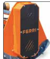
Trasmissione laterale a 5 cinghie e cofani con martinetti. Lateral 5-belt drive and hood with hydraulic cylinders.
