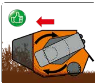
Rotore a denti fissi con riporti al tungsteno. Rotor, fixed teeth with tungsten coating and rotor with steel profiles.
