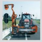
Patented hydraulic device permitting the outer arm to be litted in order to overcome possible posts, trees, obstacles.
