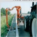
With such a system it is not necessary to slow down the working speed or stop the machine in case of overcoming obstacles. When lifted the outer blade will automatically stop while the inner one will keep on working
